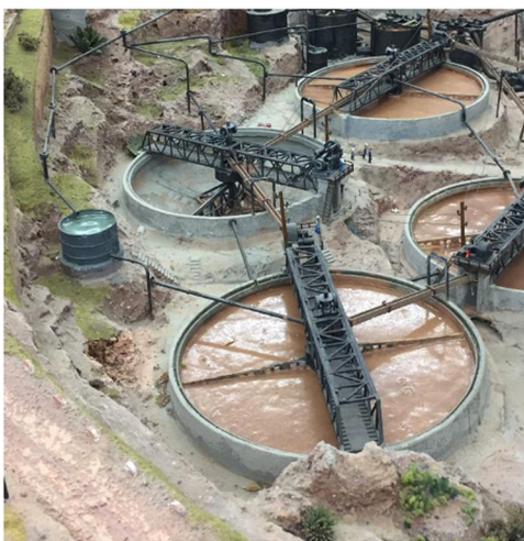
FIGURE 1 The model of mining thickeners (left) and schematic view of a bridge-type thickener (right). Fluid zones have been not-to-scale drawn
